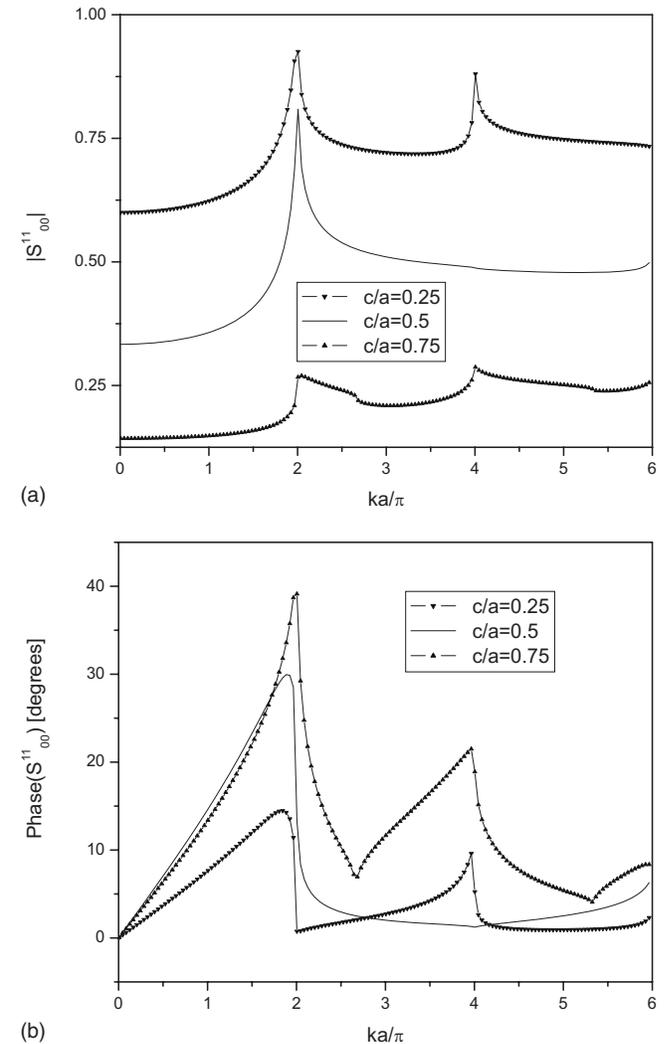
FIG. 9. (a) The magnitude of the plane wave reflection coefficient  $S_{0,0}^{11}$  for the symmetric junction in Fig. 8 with ratio of widths  $c/a=0.25$ ,  $c/a=0.5$ , and  $c/a=0.75$ . (b) The phase of the plane wave reflection coefficient  $S_{0,0}^{11}$  for the symmetric junction in Fig. 8 with ratio of widths  $c/a=0.25$ ,  $c/a=0.5$ , and  $c/a=0.75$ .
