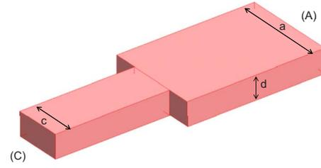
FIG. 8. (Color online) A planar junction of two rectangular waveguides of equal height.
