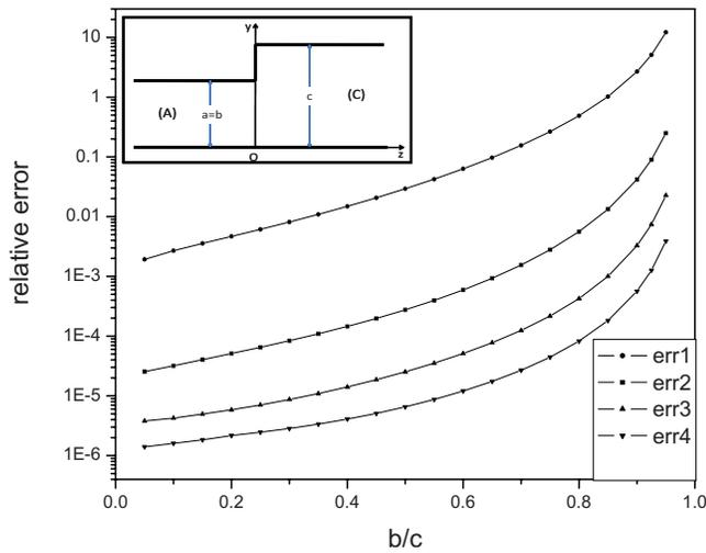
FIG. 6. (Color online) The plot of the relative errors corresponding to the cases where 1, 2, 3, and 4 equations were retained in the infinite set of equations.
