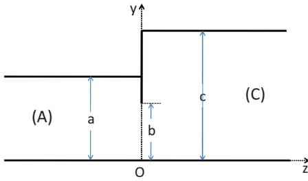
FIG. 3. (Color online) The junction between two symmetrical waveguides.
