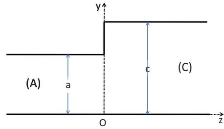
FIG. 4. (Color online) A step discontinuity in a rectangular waveguide (symmetrical case).
