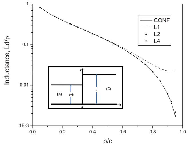
FIG. 5. (Color online) Variation of the inductance of a step discontinuity with the ratio  $b/c$ .
