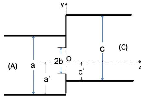
FIG. 1. (Color online) A planar junction between two general rectangular waveguides of equal width.
