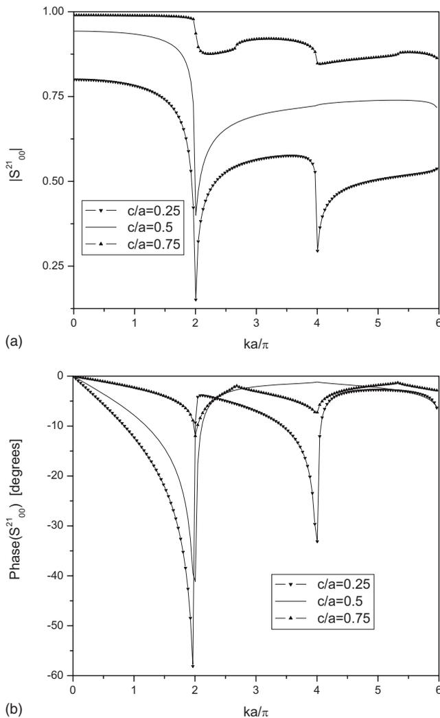
FIG. 10. (a) The magnitude of the plane wave transmission coefficient  $S_{00}^{21}$  for the symmetric junction in Fig. 8 with ratio of widths  $c/a=0.25$ ,  $c/a=0.5$ , and  $c/a=0.75$ . (b) The phase of the plane wave transmission coefficient  $S_{00}^{21}$  for the symmetric junction in Fig. 8 with ratio of widths  $c/a=0.25$ ,  $c/a=0.5$ , and  $c/a=0.75$ .
